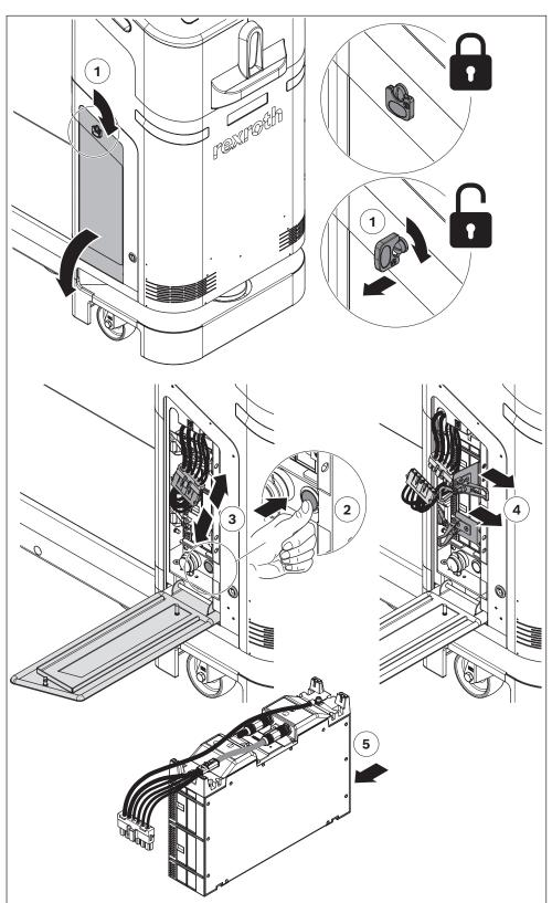
Fig. 16: Emergency measure removing lithium-ion battery
