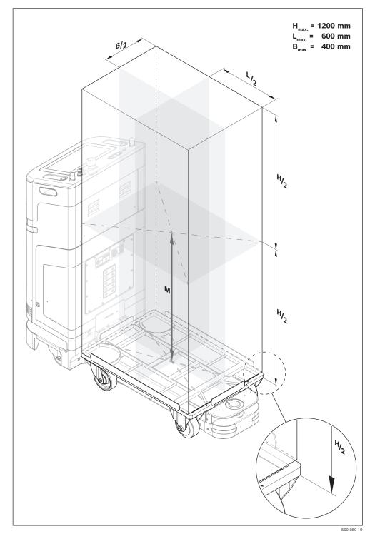
Fig. 30: Position of the mass point of the load
