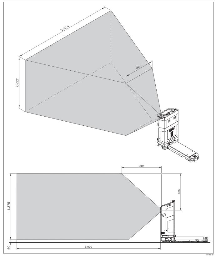
Fig. 31: Field distance range obstacle detection (all dimensions in mm)
