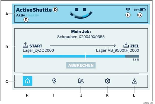
Fig. 6: Screen display ACTIVE Shuttle (shown here: job overview view)
