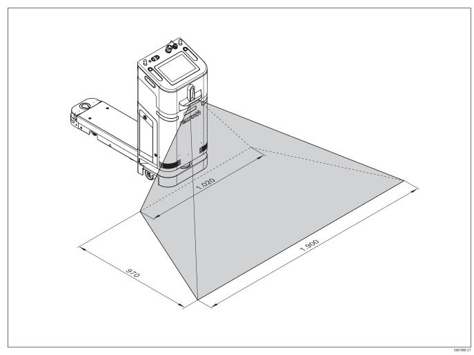
Fig. 32: Field close range obstacle detection (all dimensions in mm)
