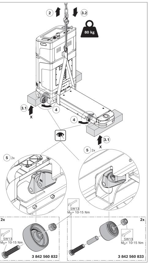
Fig. 25: Replacing the cam rollers
