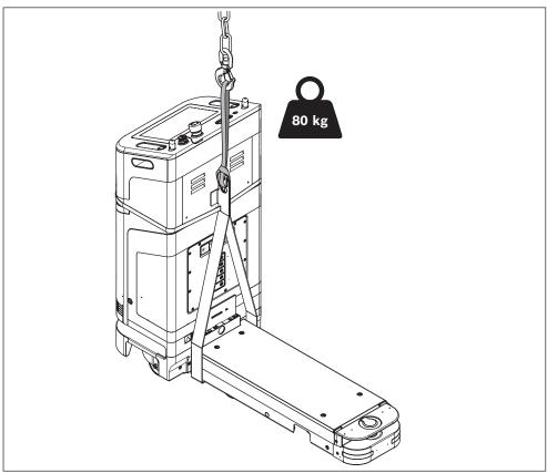
Fig. 14: Lift the ACTIVE Shuttle
