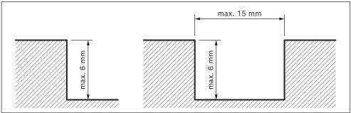
Fig. 29: Admissible uneven floors and joints
