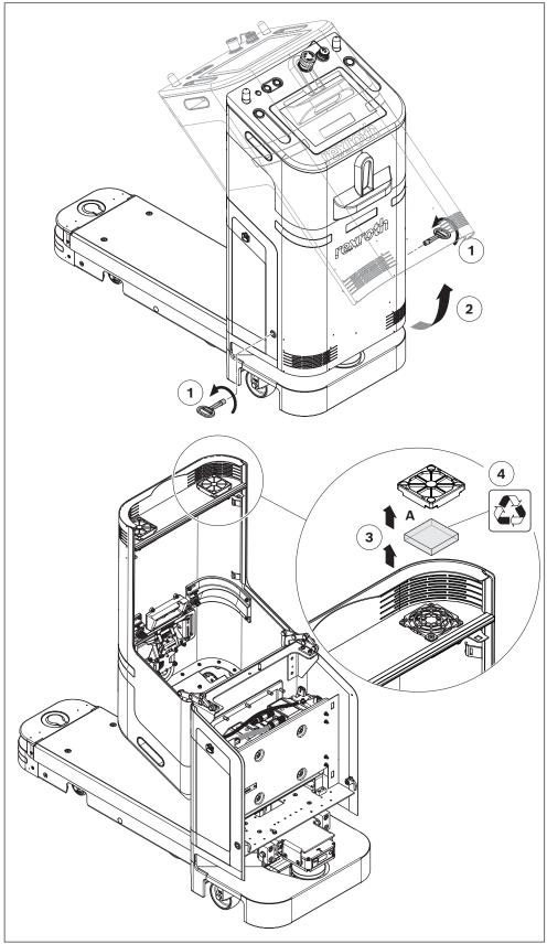
Fig. 24: Replacing the filter mats (example illustration)
