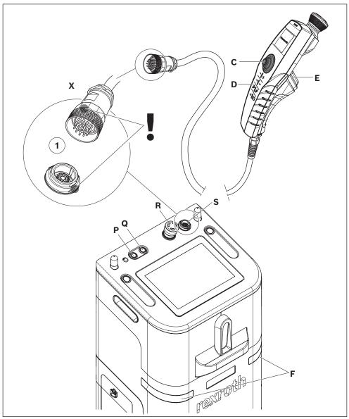
Fig. 18: Switching to "Manual" operating mode
