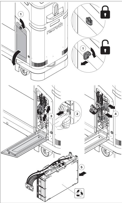
Fig. 27: Replacing the lithium-ion battery
