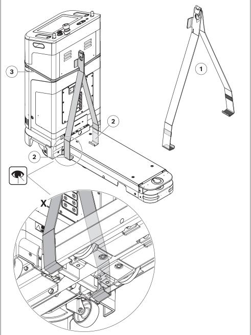
Fig. 8: Mounting/removing the lift aid
