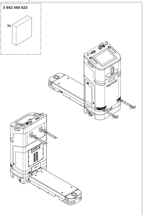
Fig. 23: Set of filter mats and fan positions
