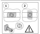
Connection with T-bolt and flange nut.
