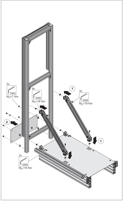
Fig. 10: Mounting the assembly frame
