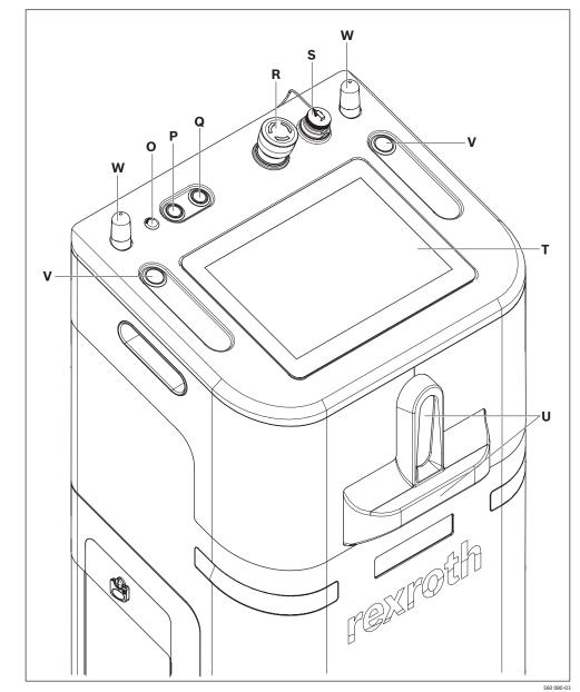
Fig. 2: ACTIVE Shuttle, detailed view of control panel
