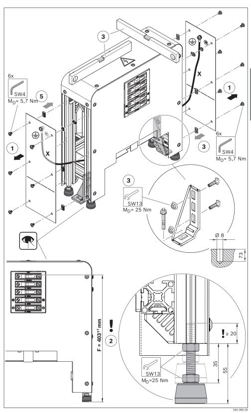
Fig. 11: Docking station assembly
