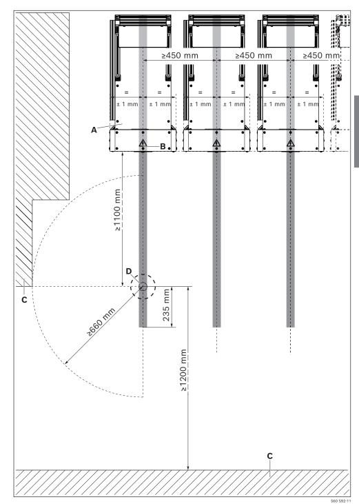
Fig. 9: Positioning the charging station
