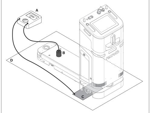
Fig. 28: Schematic diagram of the derivative value measurement
