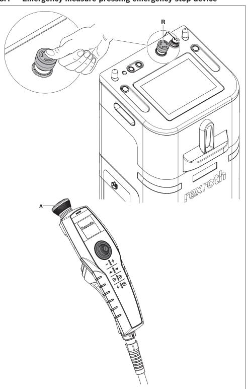
Fig. 15: Emergency measure pressing emergency stop device
