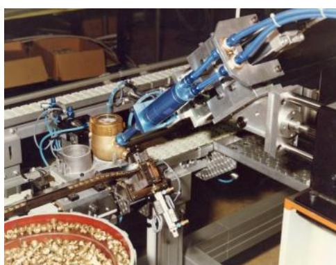
Plugs screwing station on water meters (air motor NF22424).
